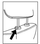
Pull the head restraint up to raise it. To lower the head restraint, press the button, located on the top of the seatback, and push the restraint down.
